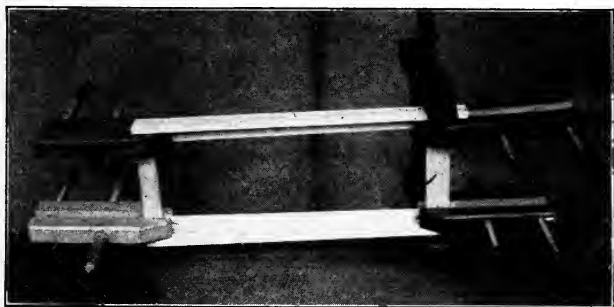
Fig. 331—Clamping Rails to Legs
